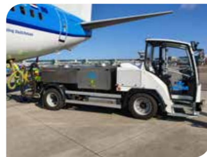
2019: Electrical water and toilet unit – The first electric Vestergaard GSE unit
