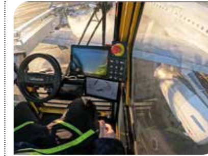
2025: OPTIM-ICE – Assisted deicing controlled by radar and camera
