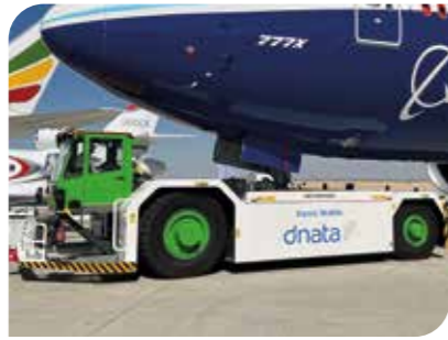
2014: TBL800 hybrid electric – The first electric tractor capable of handling the Airbus A380
