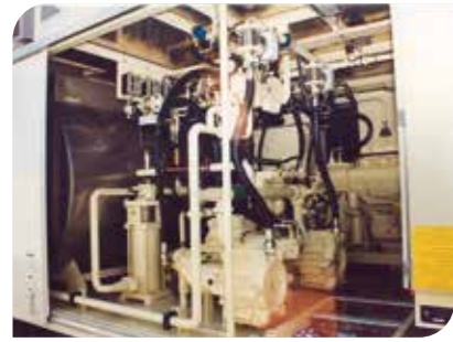
1988: Proportional Mix – Reduction in glycol consumption by mixing water and glycol directly on the vehicle
