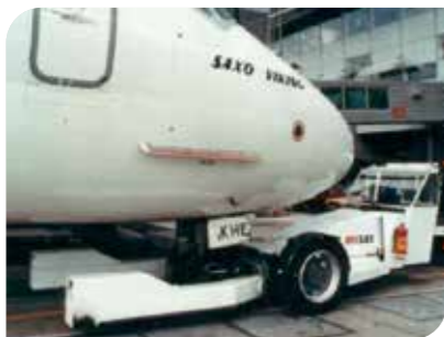
1989: Towbarless Tractor (TBL) – We pioneered the TBL – making aircraft movement easier and more sustainable
